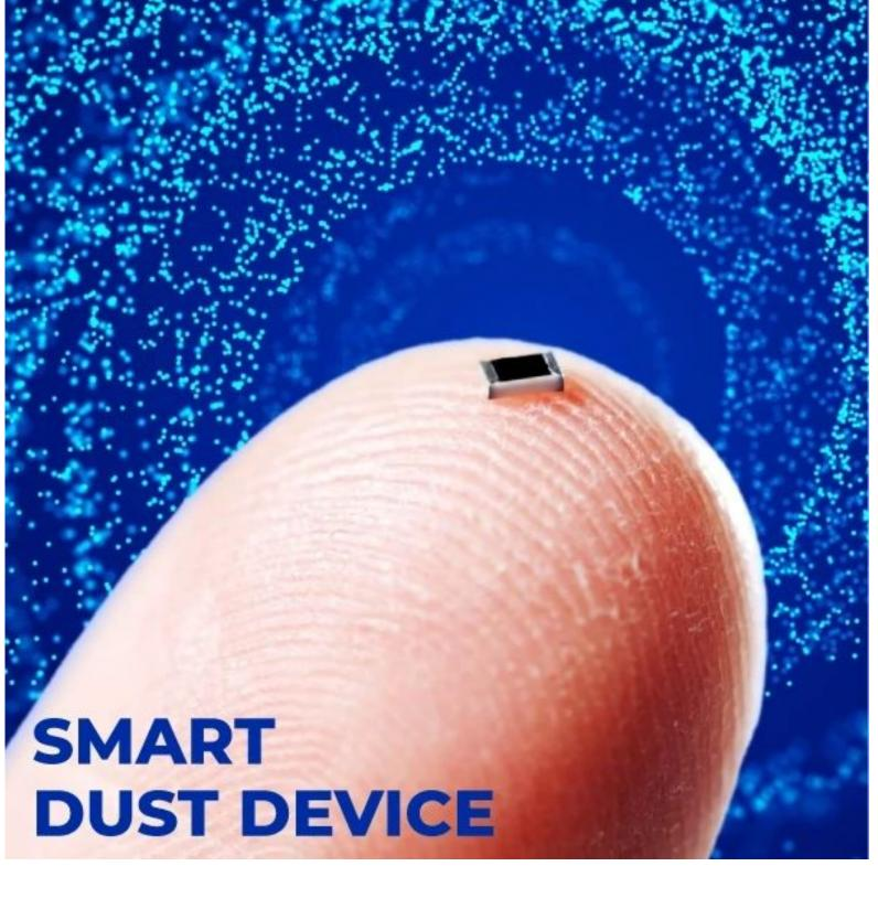
Smart dust is a swarm of tiny, wireless sensor particles, each the size of a grain of sand. They can collect data from their surroundings (light, temperature, sound, movement, chemicals, air pressure) and transmit it to a receiver without needing human control.
